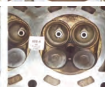
Combustion chamber after P.i. treatment.
