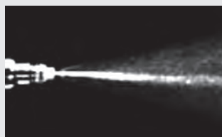
Injector spray pattern before P.i. treatment.
