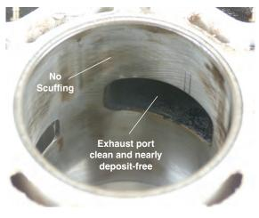
Following 534 hours in service, the cylinder bores demonstrated 0.00% scuffing and the cross-hatch pattern is 100% intact. The exhaust ports are nearly deposit-free. Results prove the superior protection and clean-burning properties of HP Marine.
